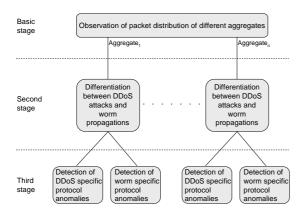
Fig. 3. System architecture for attack detection in small provider networks
