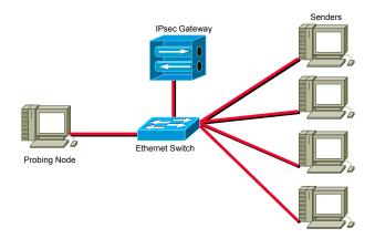
Fig. 7. The setup of the stress tests
