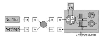
Fig. 4. A simple dispatcher configuration
