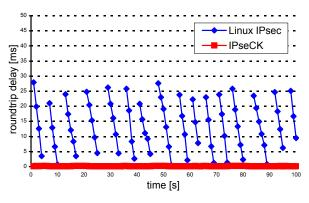
Fig. 8. Stress test with non-IPsec probes
