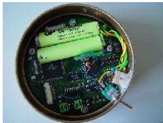
Fig. 3: “Saucer” for the flower pot with microcontroller and Bluetooth module
